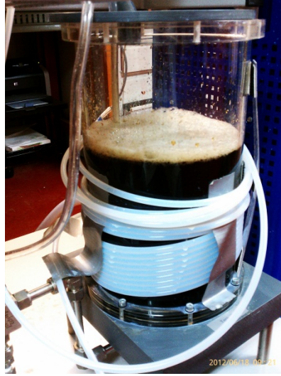
Figure 22: 8L of leachate in CE584 reservoir
