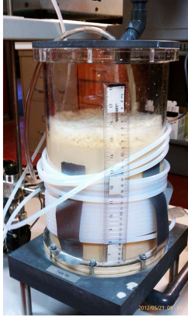
Figure 23: Leachate containing TiO 2 photocatalyst
