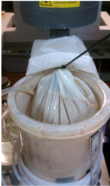
Figure 27: Nylon monofilament filter bag attached to advanced oxidation machine for catalyst recovery
